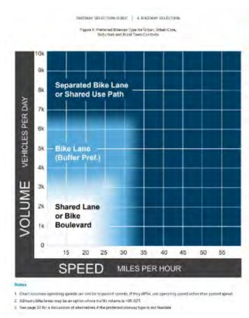
Figure 10.9 - FHWA Bikeway Selection Guide
