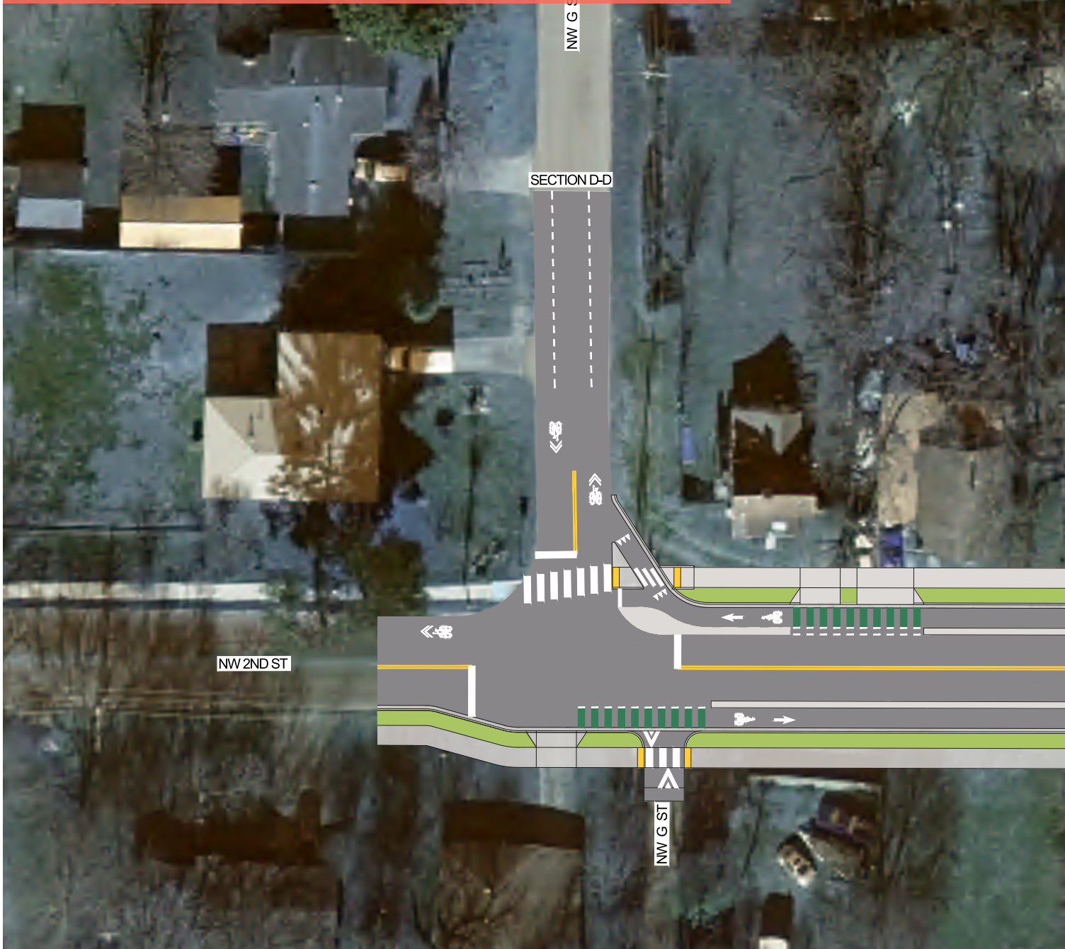
Figure 3-4: Advisory Shoulder/Directional Protected Bike Lanes - Bentonville
