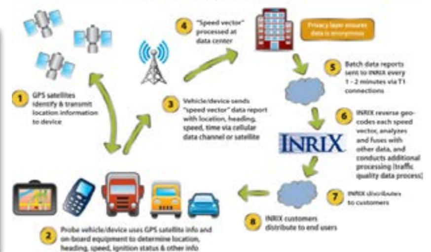
How Vehicle GPS Probe Data Works
